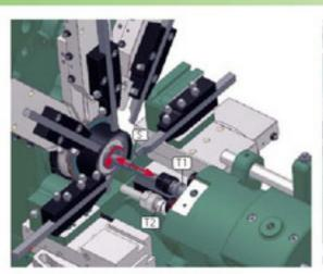
DUAL SHAFT - TAPPING SHAFT ATTACHMENT
